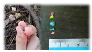
The size of microplastic that measured is fewer than five millimeters.
